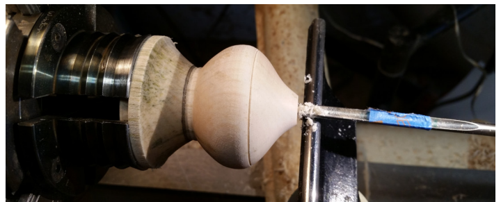
Figure 1. Shaping the exterior of the hollow form.
