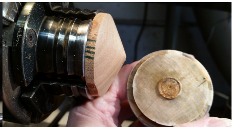
Photo 7. Jam chuck and center mark on the tenon.
