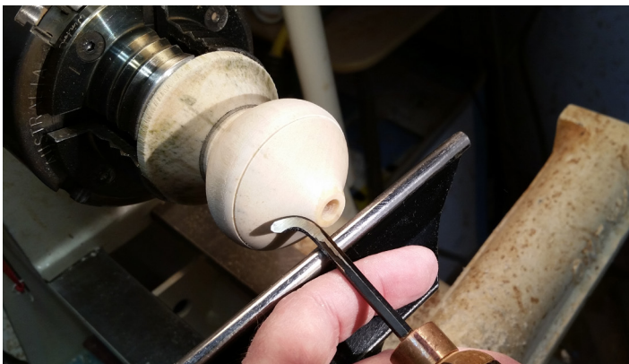
Photo 4. 90° hollowing tool, made from an allen wrench.
