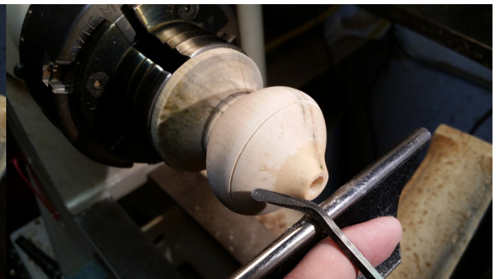
Photo 5. 45° hollowing tool, made from an allen wrench.
