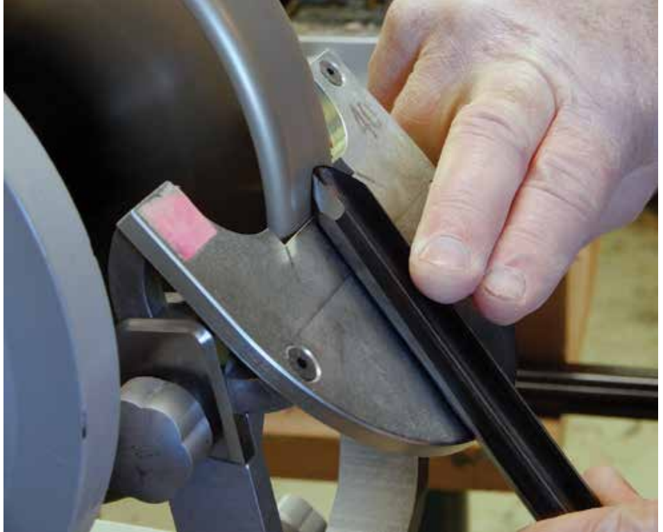
Grinding a CPM 10V particle-metal gouge on a CBN grinding wheel. Microscopic views of the grinds reveal that CBN wheels are capable of sharpening particle-metal tools to a very keen edge.
