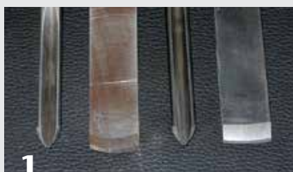
From left to right: M2 HSS gouge and scraper, and a CPM 10V particle-metal gouge and scraper. All have been sharpened with CBN grinding wheels. While conventional wisdom says we cannot get particle-metal tools as sharp as conventional HSS, with CBN wheels this is no longer true.
