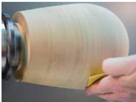
If your hand becomes uncomfortably warm from applying sanding pressure, you are turning too fast and not letting the abrasive do the work. Light pressure and slow speeds are the way to go.
