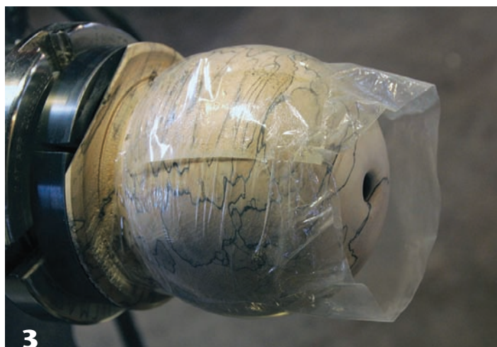
Plastic wrap traps in the wood’s moisture during hollowing, postponing evaporation until the vessel’s wall thickness is made consistent.
