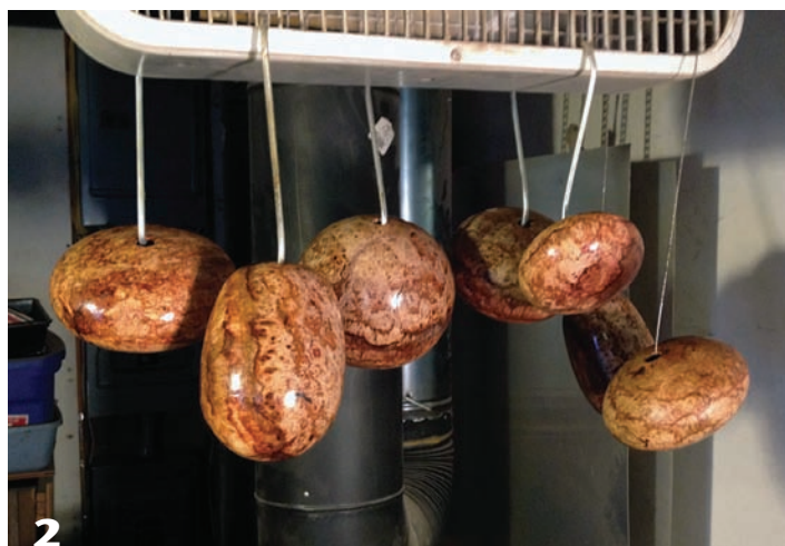
The author’s Spirit Forms drying above his woodstove. Consistent wall thickness is the key to preventing cracks in the wood.
