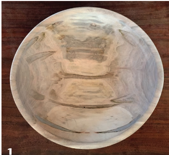
This large maple bowl went out of round and distorted significantly during drying on top of the author's woodstove but did not crack due to its consistent wall thickness.
