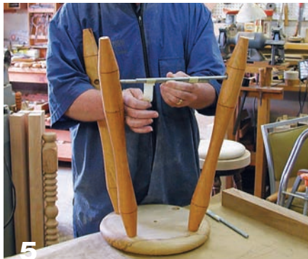
5 To get an accurate measurement for your rungs, push two sections of all-thread rod into the rung holes, then tape together the rods. The rod threads lock onto each other, preventing slippage when you remove the legs from the seat.
