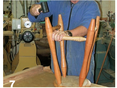
7 Use a dead-blow mallet to drive the legs into the seat.
