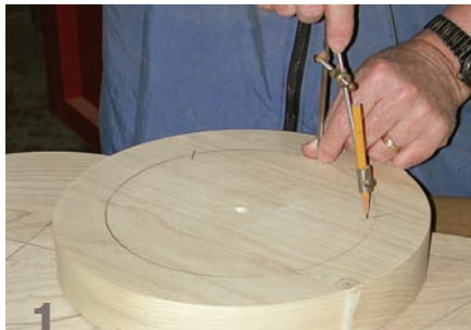
1 Using a compass, lay out the leg positions on the bottom of the stool seat.
