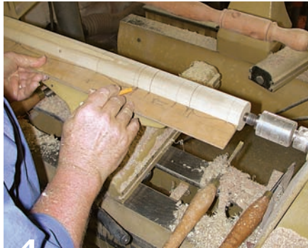
4 A pencil or marking gauge (sometimes called a story board) will help you turn four matching legs. After you've finished one leg, place the sample leg behind your lathe to use as a reliable reference.
